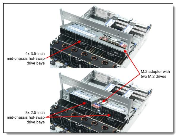
Figure 8. Mid-chassis drive bays
