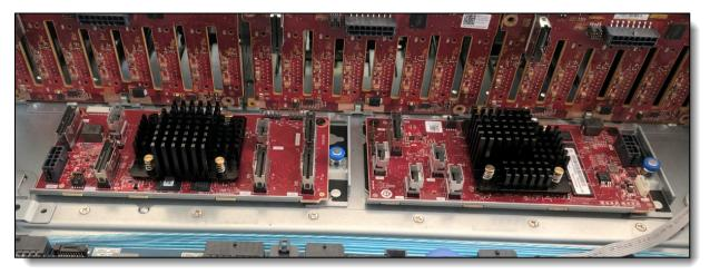
Figure 14. ThinkSystem 36i 12Gb Internal Expander (left) and ThinkSystem RAID 940-16i Internal Adapter (right) installed in the ThinkSystem SR665 (cables and system fans removed for clarity)
