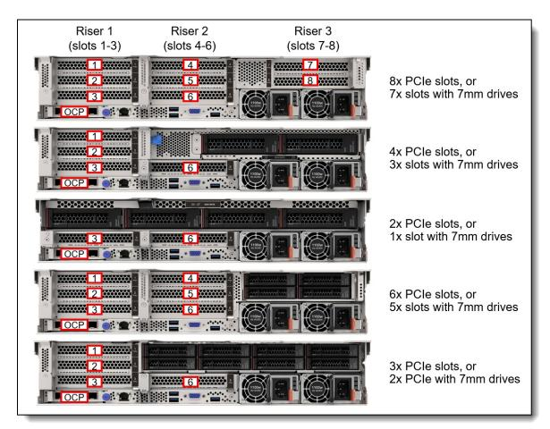
Figure 15. SR665 slot configurations
