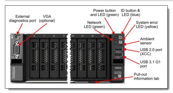
Figure 18. Front operator controls are on the left and right side of the server
