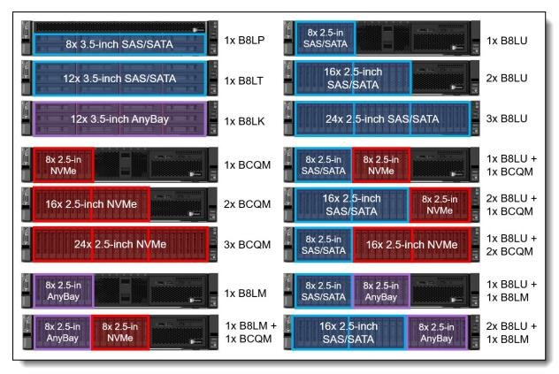
Figure 7. SR665 front drive bay configurations
